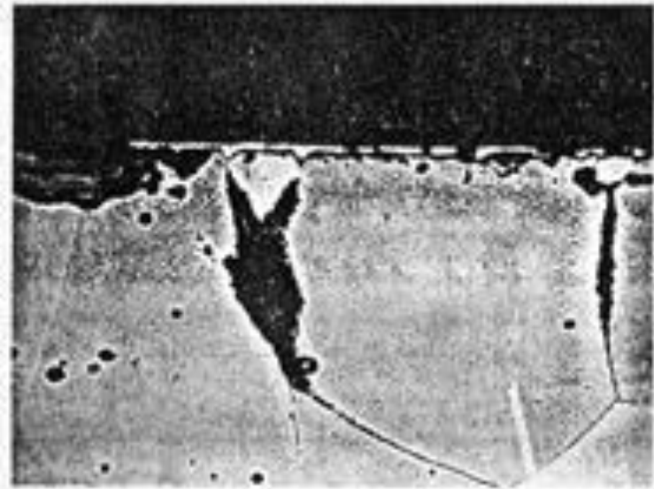
Figure 30.55 Photomicrograph of an etched cross section removed from a tab underneath the base of the Loma Negra seated man illustrated in figure 30.20. Note the large grain size of the annealed copper, the spherical oxide inclusions, and the grain boundary corrosion. At the surface of the copper sheet the electrochemically deposited gold layer is just visible.
