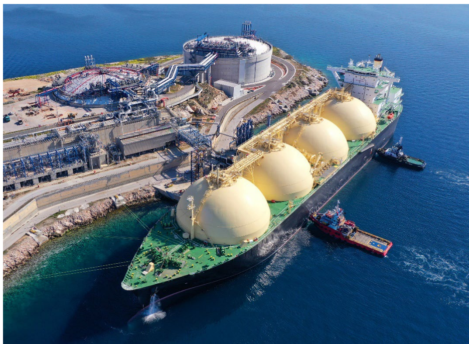
FIGURE 3. This example of an LNG tanker docking at an LNG ship terminal shows how the tanker resembles a hollowed-out oil tanker or container ship with the oil tanks or container holds replaced by well-insulated spherical LNG tanks. Source: Aerial-motion/Shutterstock.com
