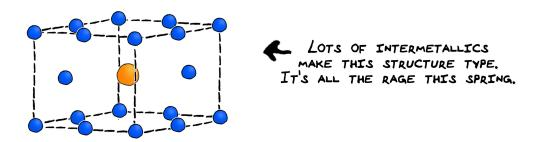
We call it "The CaCu $_5$  type", which doesn't mean that it absolutely has to contain calcium or copper, it just means that the first time we saw this structure, that's what we happened to be looking at. The essence of the CaCu $_5$  type is the specific atomic positioning.
