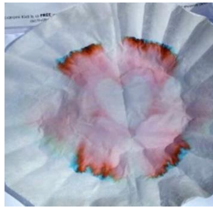
Figure 7. Illustration of separating proteins by chromatography (top). Proteins bind to the carbon with different strengths. As liquid is added and it washes the proteins off the solid. The proteins that interact the strongest stay on longer while the proteins that interact less come off first. A common demonstration of this is separating dyes using a coffee filter (bottom). As you can see, different dyes migrate more or less once the liquid is added. The different colors separating from each other based on the strength of their interaction with the filter.
