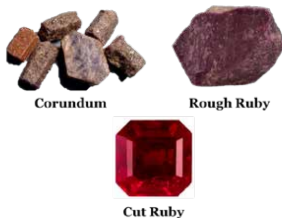
Figure 1.3 The mineral corundum is composed of aluminum and oxygen. Upon introduction of a chromium impurity, a ruby can be formed. Both a rough ruby and cut ruby are shown for contrast. 4
