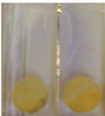
Figure 4. The quaternary phase \text{Cu}_2\text{Bi}_3\text{Sb}_3\text{O}_{14} on a glass slide after removal of excess residue from the heating process.
