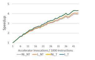
(a) Simulator-based estimation of tightlycoupled accelerator speedup.
