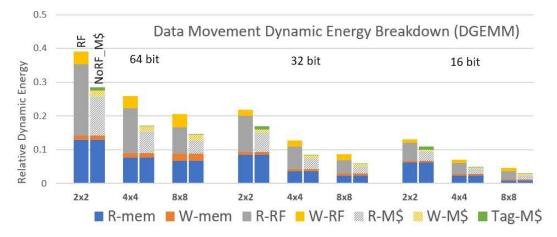
Figure 1.3: Energy consumption moving data in tightly-coupled accelerators using the old method of the Basket/RF (left bar per pair) compared to using our proposed method (right bar per pair). Lower is better. Overall height is decreased for every pair, showing a reduction in energy consumption, which is good.
