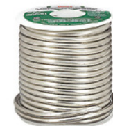
This lead-free solder is 94 percent tin and 6 percent silver.
