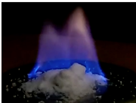
Figure 3. This image of the flame from ignited methane hydrate (white solid) is from a YouTube video, “ Burning Ice - Fire Ice - Methane Hydrate - (Dark room settings) ”.
