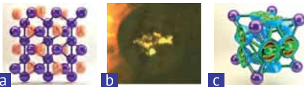
Examples of unusual forms of matter formed under pressure: a) structure and b) optical microphotograph of transparent form of sodium; c) structure of non-conventional compound \text{NaCl}_3 .
