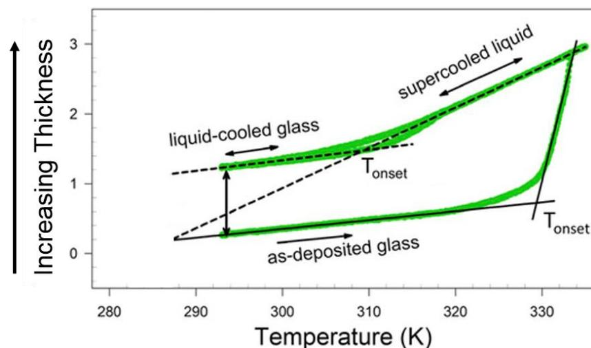
Figure 5. Percent thickness change upon heating of a vapor-deposited glass (bottom curve) and a liquid-cooled glass (top curve). Note that the onset temperature of the as-deposited glass is significantly higher than the onset temperature of the liquid-cooled glass. Reproduced with permission from Ref. [2].
