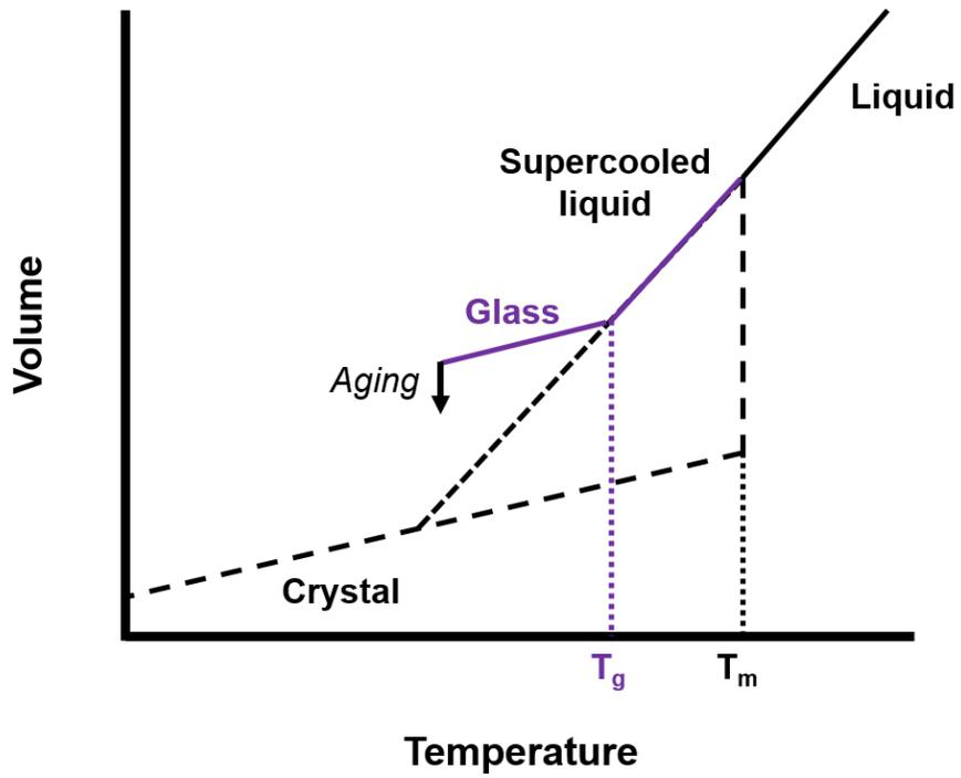
Figure 2. Volume as a function of temperature illustrating how a glass is typically prepared. The arrow indicates aging, as the glass is continually trying to reduce its volume.
