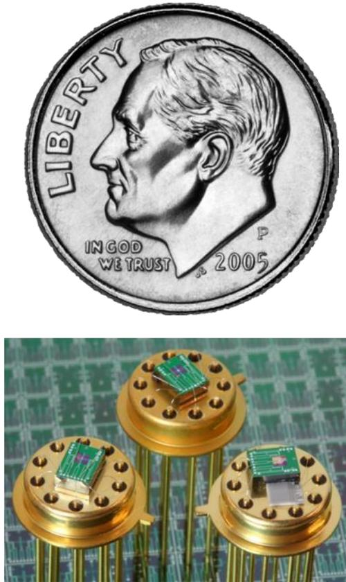
*Figure 6. Nanocalorimeter devices shown against a dime for scale. The green chip on the top of the device contains the 30 micron square active area that is actually used for a measurement. The width of the active area is equivalent to the diameter of a thin human hair and requires only nanograms (one nanogram = one billionth of a gram) of material for analysis. Figure courtesy of [xensor.nl](http://xensor.nl).*
