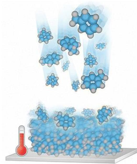
*Figure 3. A schematic illustration of physical vapor deposition. After the gaseous molecules bounce around inside the vacuum chamber they will eventually find the substrate held at a particular temperature. With continued deposition a thin film made up of the deposited molecules will eventually form. Reproduced with permission from Ref. [1].*
