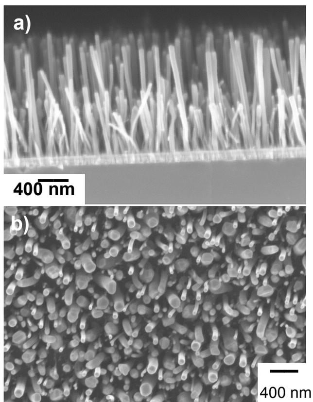
Figure 1: a) Side view of the carbon nanofibers showing their high surface area
