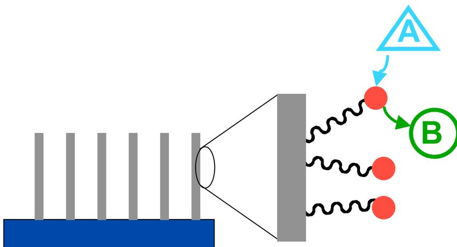
Figure 2: Diagram of the target assembly. The carbon nanofibers are depicted in grey. In the expanded section, the catalyst molecules are depicted as red circles, attached to the nanofibers by the black squiggles, which represent the molecular linker. The catalyst on the surface would take reactants (A) and convert them to products (B) while remaining immobilized.
