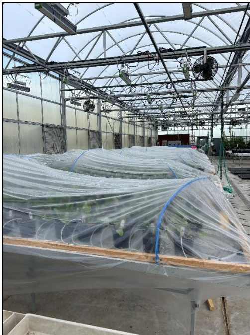
Figure 5.9. Humidity chamber construction used in linkage mapping inoculation screens. Photo taken by Audrey Morrison.
