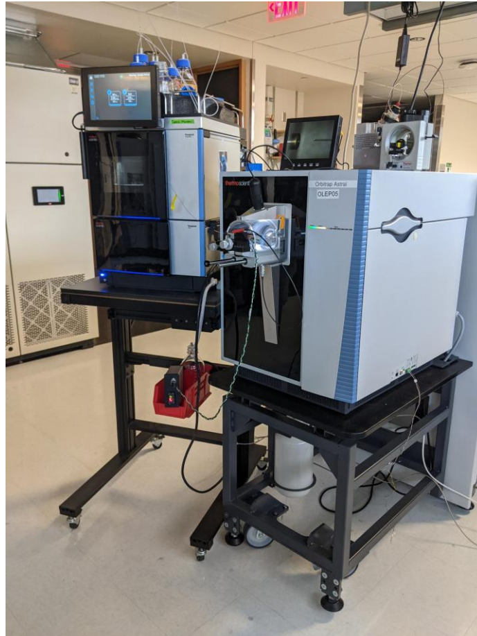
Picture 4.2: A liquid chromatography instrument (left) attached to a mass spectrometer (right). This MS instrument stands approximately 55 inches tall and weighs 1,600 lbs. Image credit: Corinne Moss
