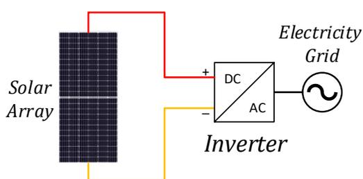
Fig. 1.8. Solar array connected to the electric grid
