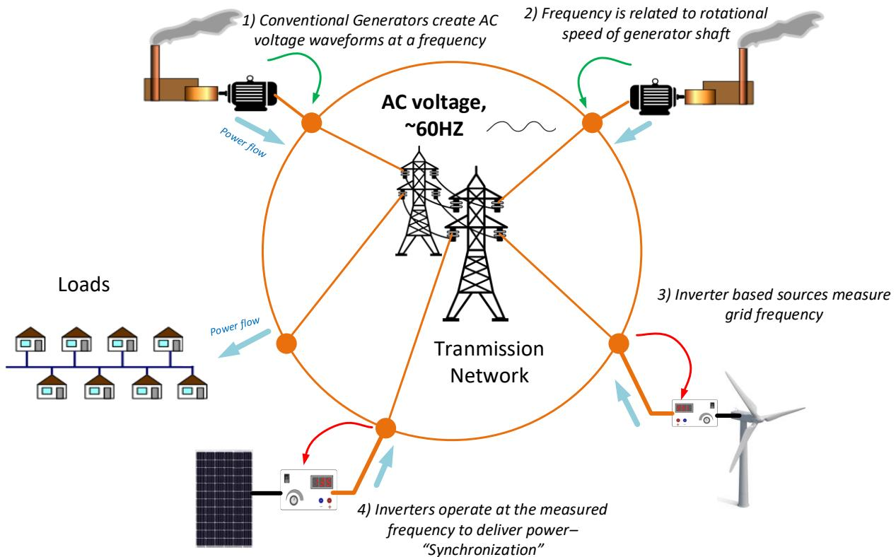
Fig. 1.10. Synchronization of Inverter based resources
