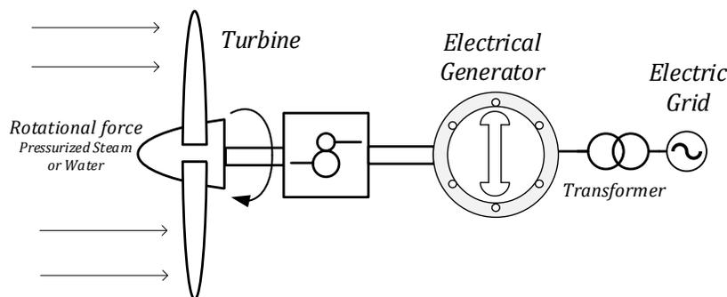
Fig. 1.5. Basic diagram of a conventional power plant
