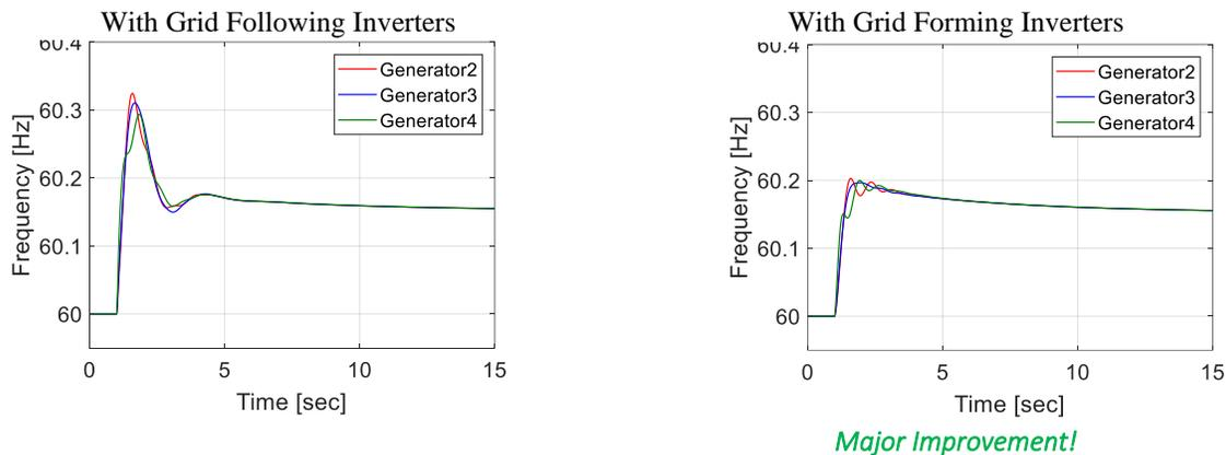
Fig. 1.15. Generator Frequency response at ~70% inverter penetration
