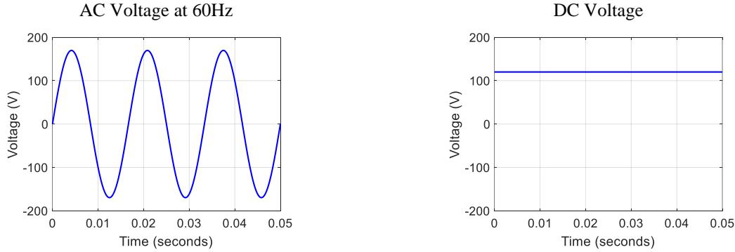
Fig. 1.3. AC vs DC voltage waveforms
