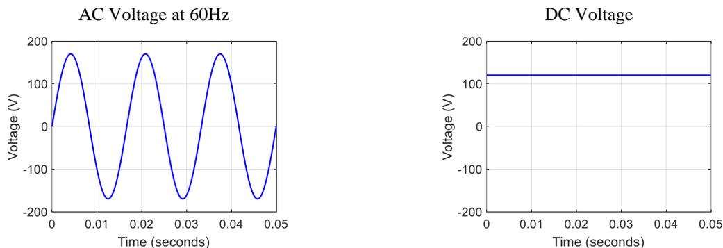
Fig. 1.3. AC vs DC voltage waveforms
