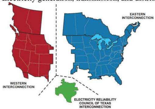
Fig. 1.2. Electric interconnections that span the United States, large parts of Canada, and a small part of Mexico
