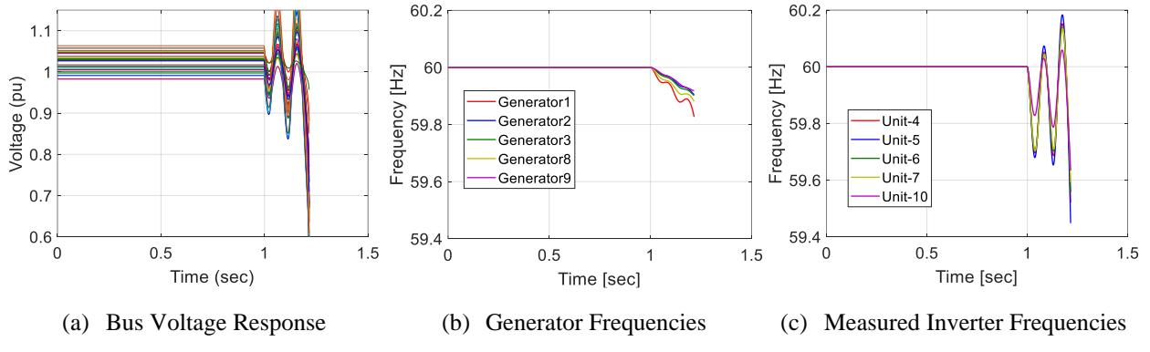
Fig. 1.12. Simulated waveforms for ~50% renewable penetration
