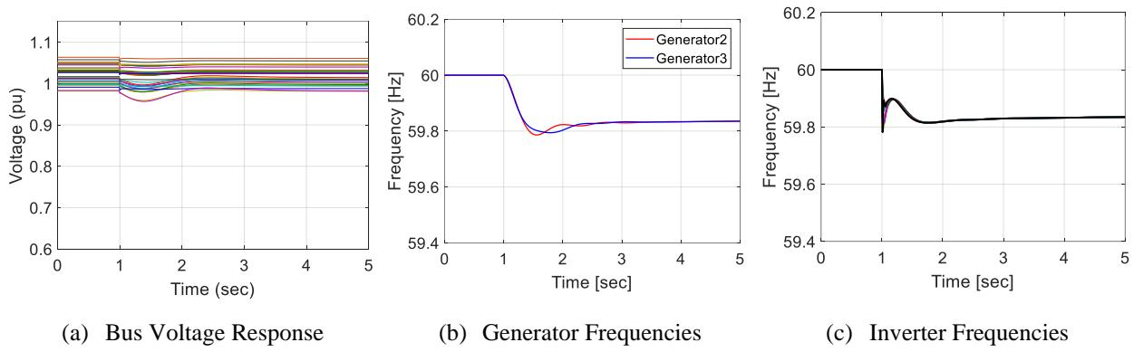
Fig. 1.14. Simulated waveforms for ~80% renewables operating as Grid Forming Inverters
