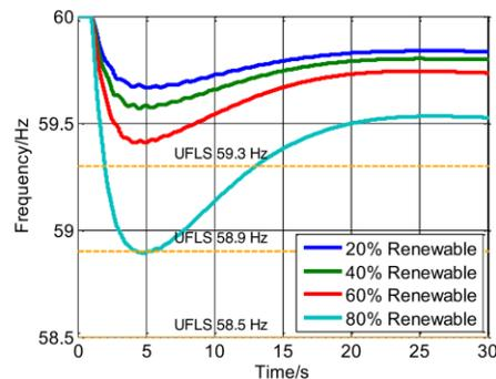
Fig. 1.11. Simulated grid frequency response at increasing levels of renewables [11]
