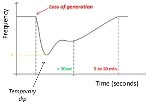
Fig. 1.6. Typical grid frequency response to a loss of generation event
