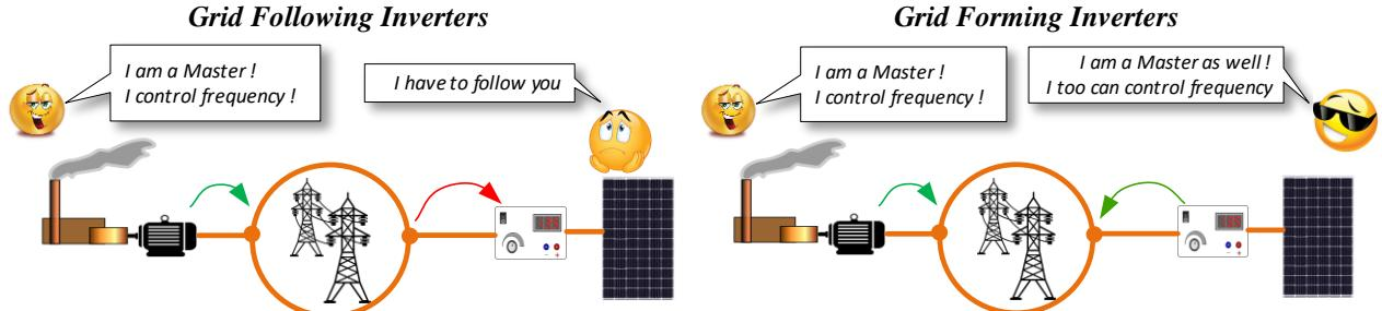
Fig. 1.13. Synchronization of Inverter based resources
