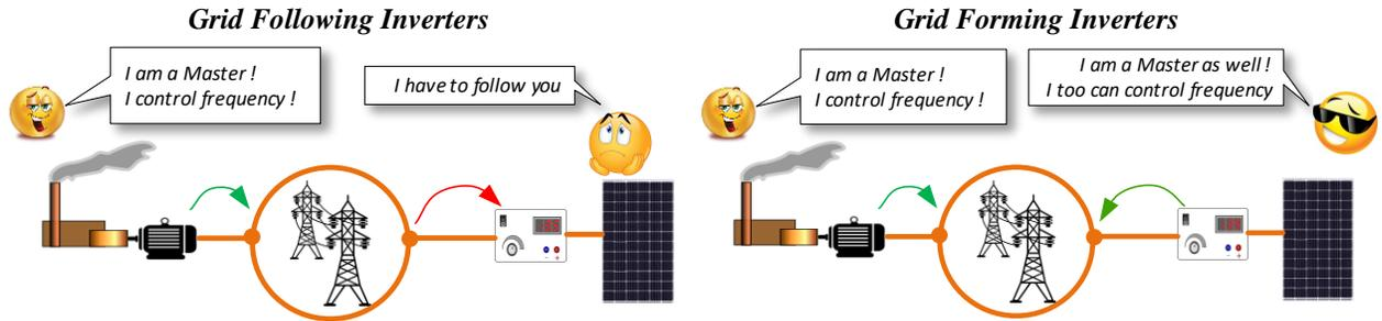
Fig. 1.13. Synchronization of Inverter based resources
