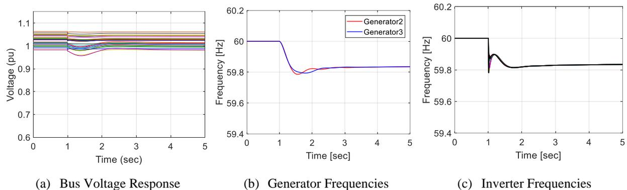
Fig. 1.14. Simulated waveforms for ~80% renewables operating as Grid Forming Inverters
