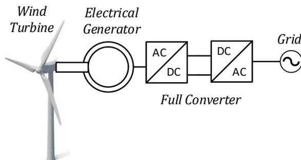
Fig. 1.9. Wind turbine connected to the electric grid
