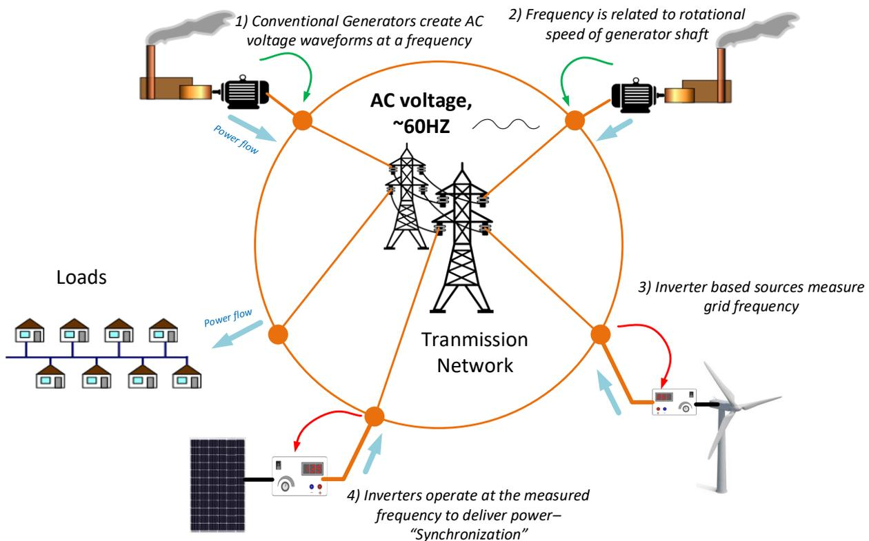
Fig. 1.10. Synchronization of Inverter based resources
