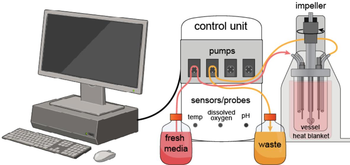
Figure 3. Schematic representation of the chemostat system with inputs and outputs labeled.
